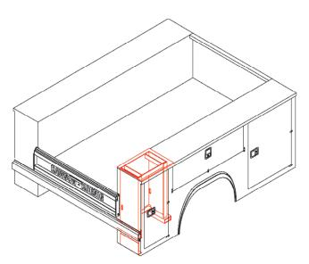
To accommodate rear corner mounted cranes with capacity to 4,000 lbs (16,000 ft. lbs.) when mounted on standard U, J, L, S, T and E-Series. Crane reinforcing is now designated in the body model part number, so CRK kit part numbers are no longer required. To designate the side of the body to be reinforced, put a C in place of the door configuration number for the appropriate side of the body (ie: L60DW1C94). Generally, bodies are crane reinforced on the curbside.
