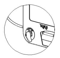
SWITCH ASSEMBLED TO BRACKET
